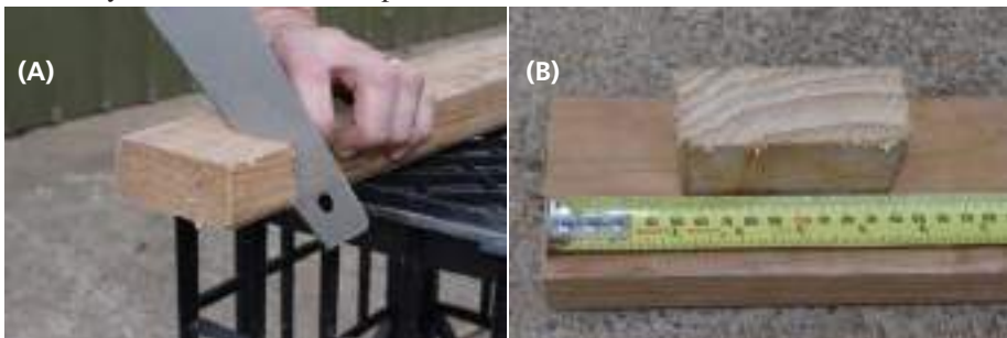
Figure 2. Demonstration of basic sample cutting with a hand saw (A) and resulting sample size (B).
