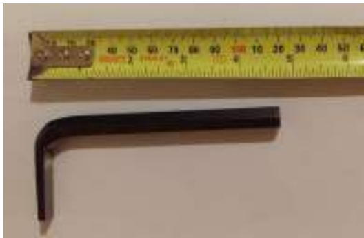
Figure 4. Example tool suitable for levering cut sample away from body of timber. The short, flat edge of the tool can be hammered into the cut groove once the drill bit has been removed and then used to lever sample away from the item.
