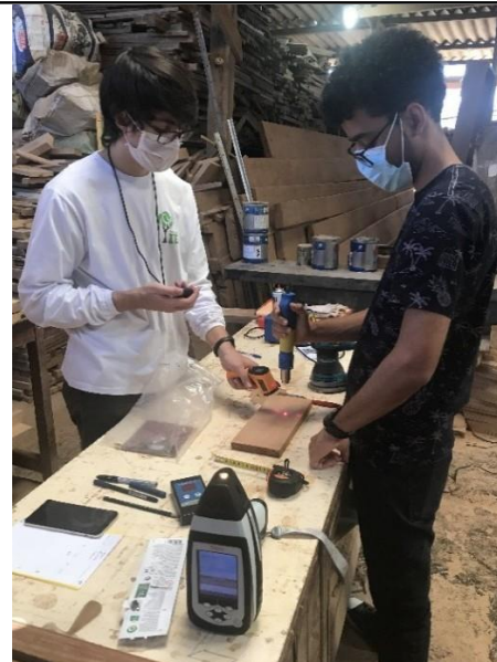
Fig.21. Applying drying protocol on samples for NIR spectra collection.
