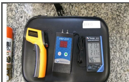
Fig.03. Digital infrared thermometer, wood moisture meter, and ambient humidity and temperature meter.
