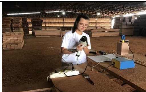
Fig. 38. Collection and reading of spectra using the NIR equipment.
