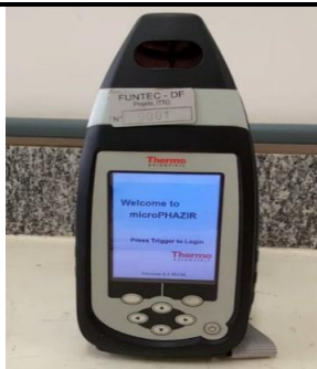
Fig.06. Microphazir equipment for reading spectra on samples.
