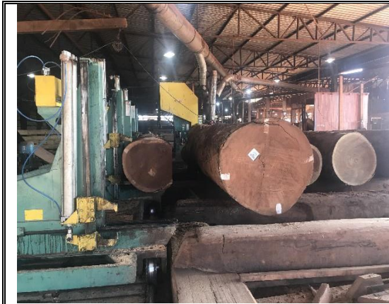
Fig.30. Beginning of log sawing.
