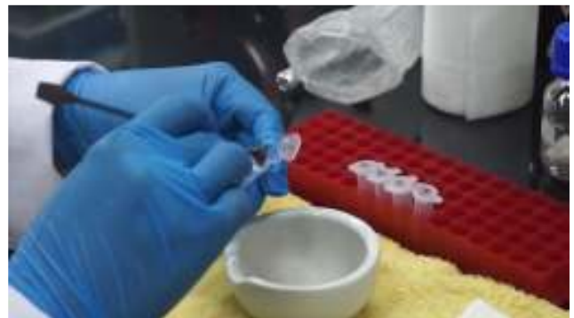
Transferring the fine powder to a 1.5 ml micro-centrifuge tube
