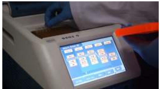
Putting the sample for amplification into a thermal cycler
