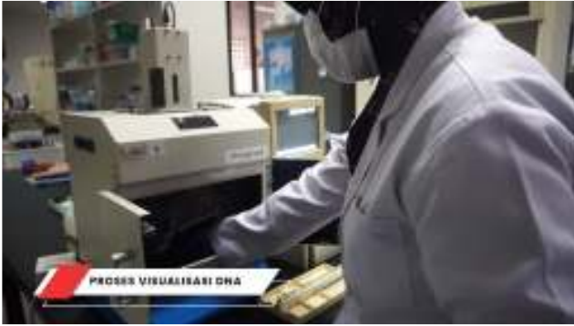
Visualization of the gel electrophoresis results using the gel documentation system
