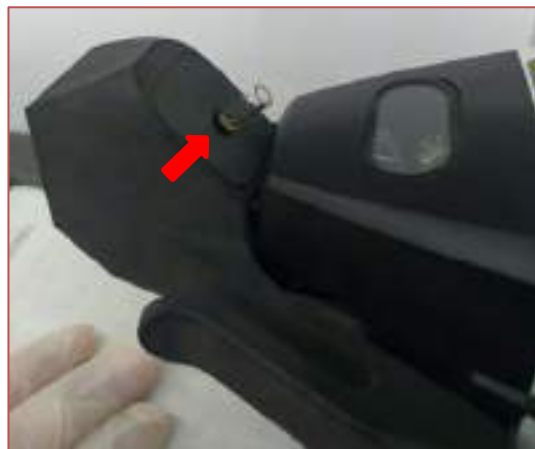
Figure 6 - Correct positioning of the vial in the accessory compartment.
