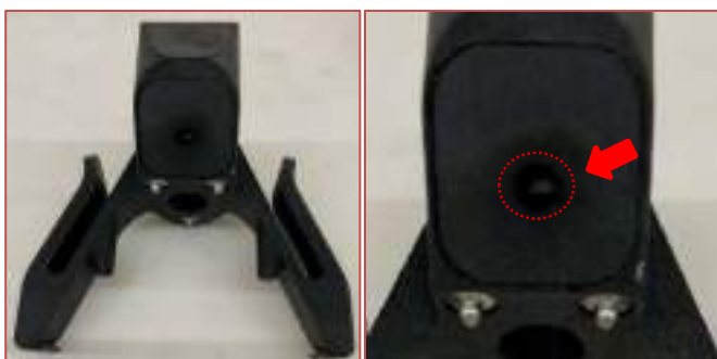
Figure 1 - Accessory of the MicroPHAZIR portable instrument for liquid analysis.
