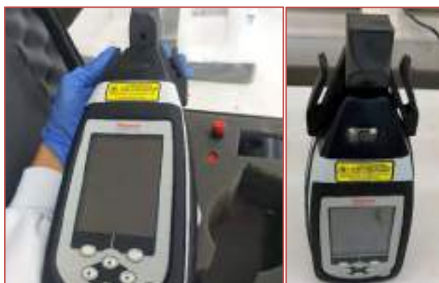
Figure 2 - Attaching the accessory to the MicroPHAZIR.
