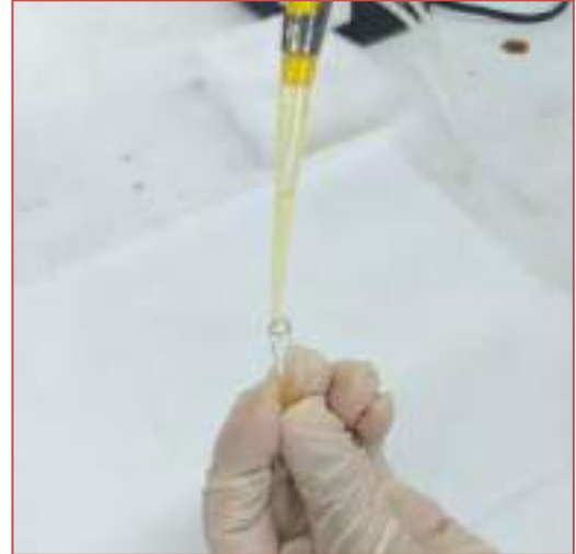
Figure 5 - Addition of the oil in the vial with a micropipette.
