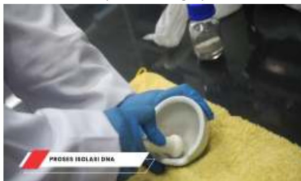
Figure 2. Grounding the wood sample to a fine powder using a mortar and pestle
