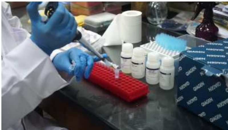
Figure 7. Transferring the supernatant to a new microtube
