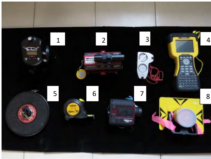
Figure 13. Mapping equipment used to determine site boundary and planting holes. 1. Angle encoder. 2. Laser range finder. 3. Tandem compass. 4. Data controller 5. Diameter tape. 6. Measuring tape 7. Handheld laser range finder. 8. Prism reflector.
