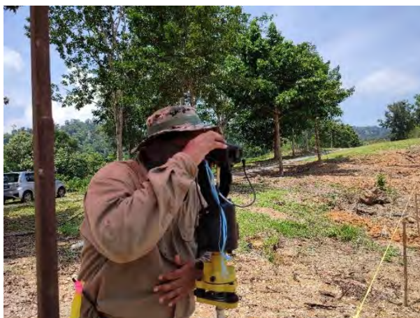
Figure 14. A temporary base station is put up as a starting point to align the boundary and planting holes.
