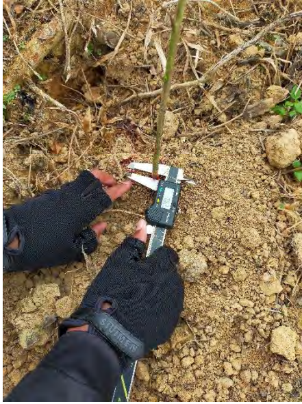
Figure 21. Diameter at the root collar is measured just above the natural ground line.
